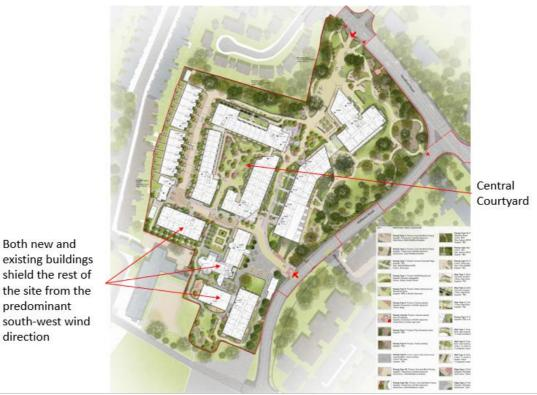
Figure 17.25: Wind Mitigation Measure – Apartment Block Arrangement
